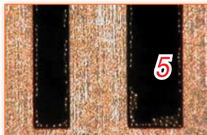
Photo 5 shows the same stencil after 20 printing cycles, wiped dry with Micro•Wipe FP paper. There are no clogged apertures, no loose fibers and no excess solder paste. This and other tests proved it is feasible, fast and reliable to wipe stencils without using solvents. This capability is available only with Micro•Wipe FP paper.
