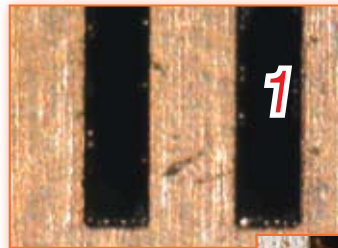
Photo 1 shows the test stencil after cleaning with Sontara® "E" paper, 20 printing cycles, wiping wet with IPA. This is an excellent "benchmark" result: clean aperture, no fibers, no excess solder paste.
