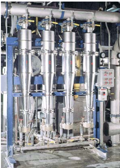
Centrifugal cleaners on the 4-cylinder paper machine.
