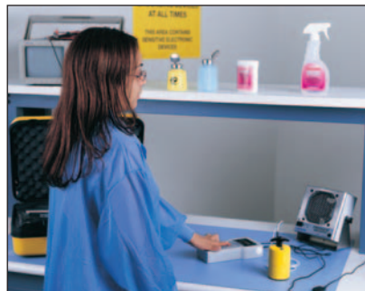
Figure 6: ESD mat with test kit
