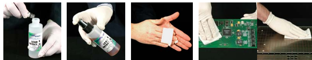
Pour one vial of Detecting SR Powder #1 into Developing Solution #3 spray bottle. Shake well to mix. Use normal hand washing pressure. Use only one side of the wipe, thoroughly wipe a designated area. Wipes may be used on irregular surfaces.
